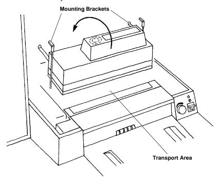
5. Lift the DSA assembly straight up from the transport area.
